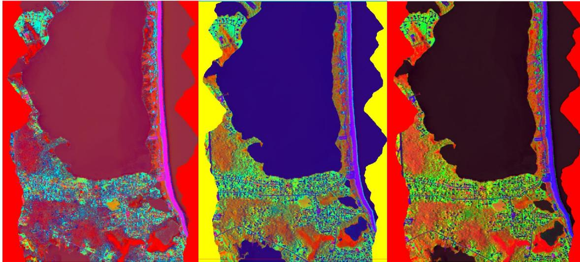
*Figure 7: False color RGB images of Ninigret Pond using SMA results from image endmember only trial (left), library endmember only trial (center), and endmember combination trial (right). Red is in the senesced vegetation band, green is in the live vegetation band, and blue is in the dry sand band.*
